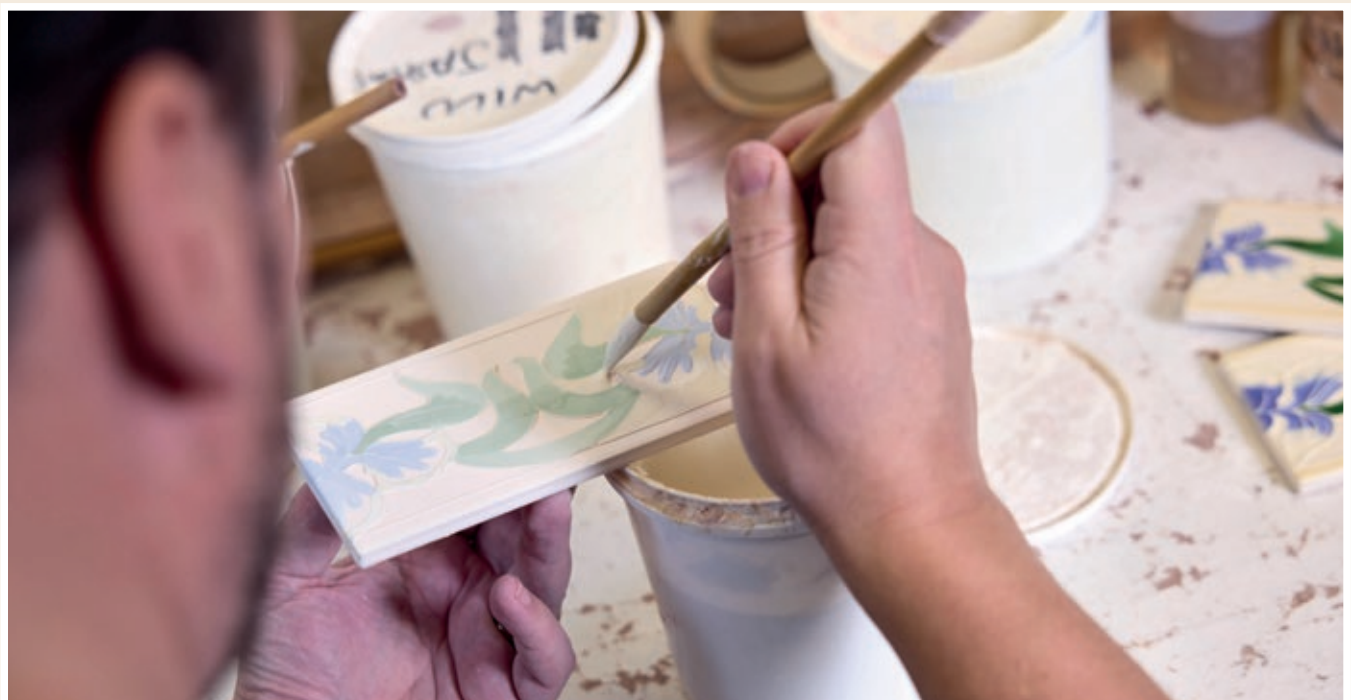
▲ When the piped outline has dried, coloured glazes are hand painted in separate areas within the lines. As you can see, the glaze colour does not resemble the finished tile
