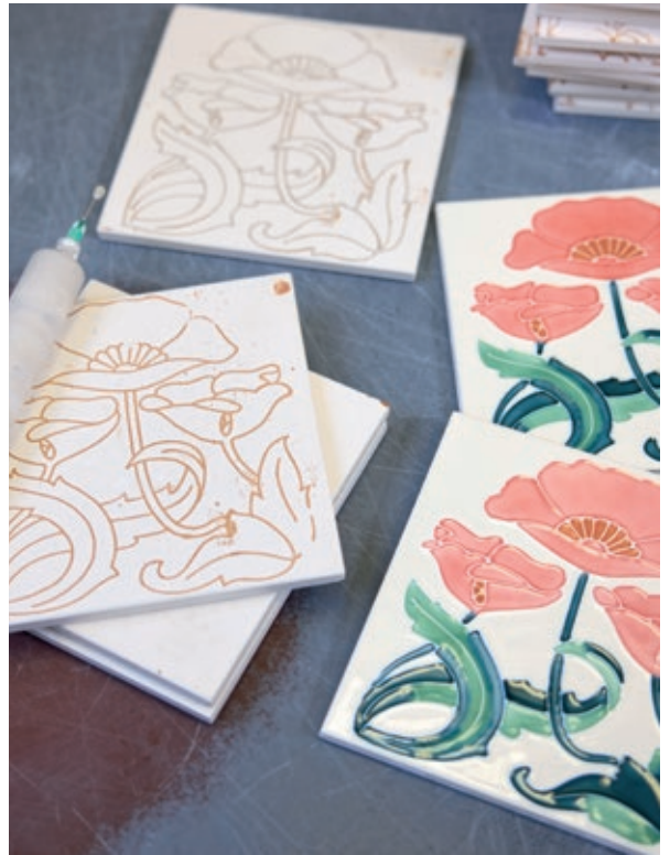
▲ Tube lined tiles before and after decorating
