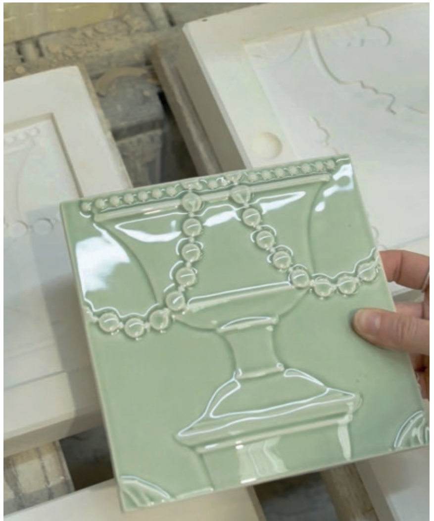
▲ Bespoke glazed moulding with plaster moulds
